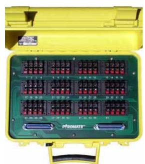
The Pyromate P-45 pyrotechnic firing system provides the ability to individually apply an activating voltage to 1 to 45 separate circuits. The 24 volt power source is internal to the control panel and is recharged thru the charge jack using a 12 VDC external power supply.
